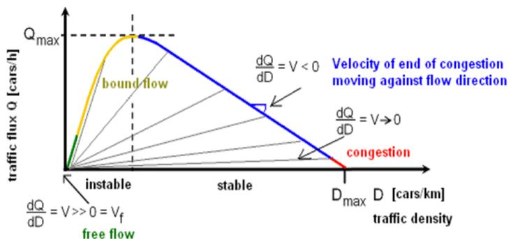
Fig. 1 Fundamental Diagram of Traffic Flow
