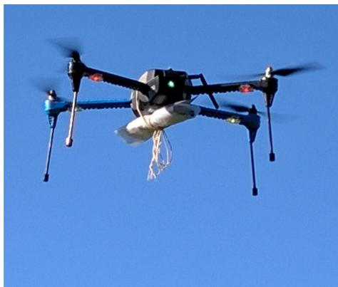
Figure 3.8: IRIS+ hovering with different payloads.
